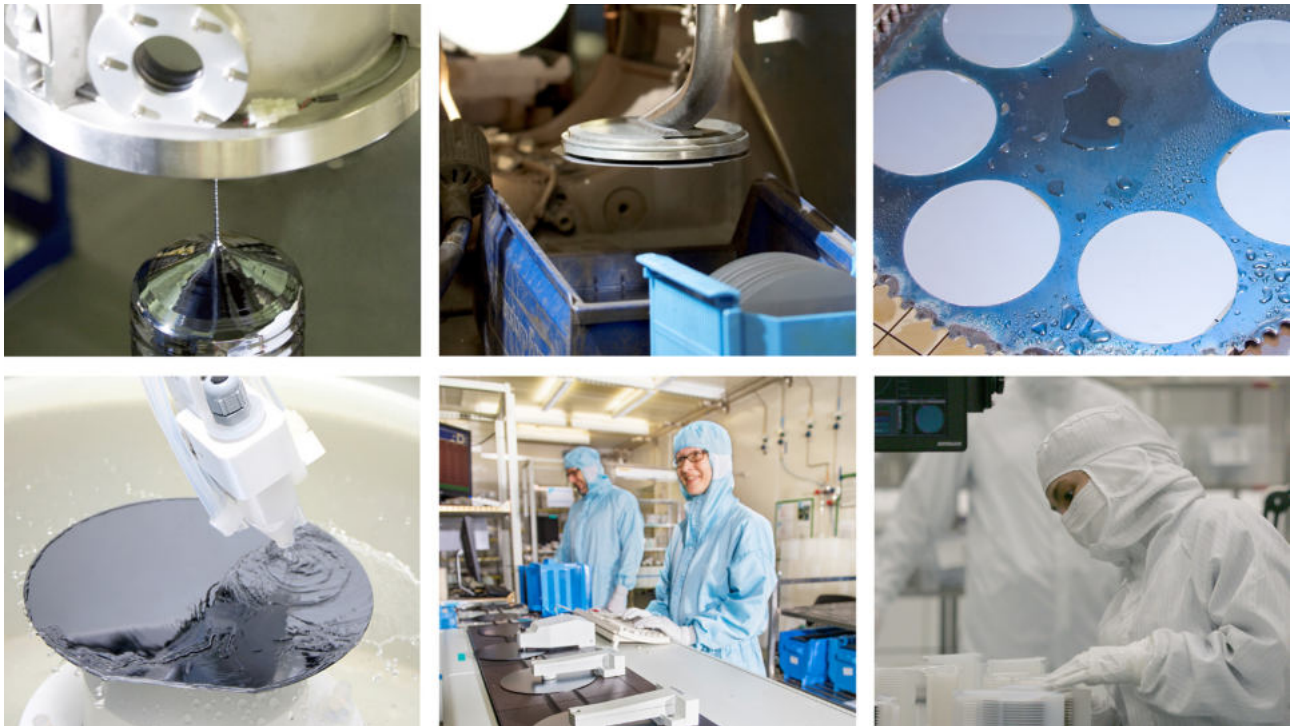
Making silicon wafers.
