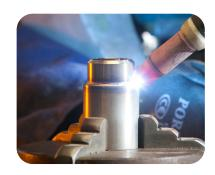
• made of a specific non-ferrous alloy with a melting point lower than the base metal. In this case the filler metal must be compatible with the base metal and must have the strength required to do the job.
