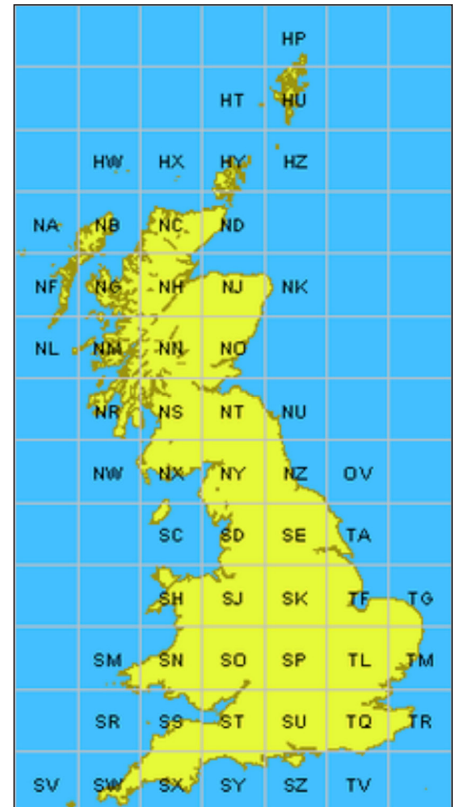
The Ordnance Survey maps of Great Britain use the Ordnance survey National Grid
