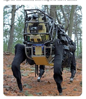
surfaces that would defeat wheels. The legs contain a variety of sensors, including joint position and ground contact. BigDog also features a laser gyroscope and a stereo vision system.
