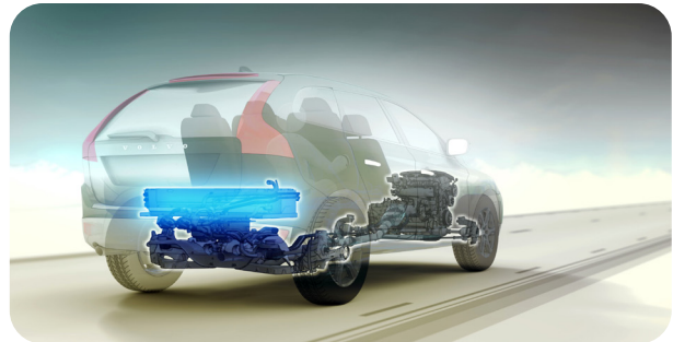
Volvo XC60 concept battery pack
