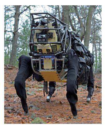
too rough for conventional vehicles. Instead of wheels, BigDog uses four legs for movement, allowing it to move across surfaces that would defeat wheels. The legs contain a variety of sensors, including joint position and ground contact. BigDog also features a laser gyroscope and a stereo vision system.
