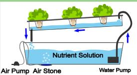
• Due to its simple yet effective design, the **Nutrient Film Technique** system (or **NFT** system) is quite popular with hydroponic growers. This versatile system is often used to grow smaller and quick growing plants like different types of lettuces, herbs, baby greens and strawberries. Two are its main components: the grow tray (or channel) and the reservoir that contains water and nutrients. In the grow tray, net pots with growing media (perlite, coconut, Rockwool) hold the plants
