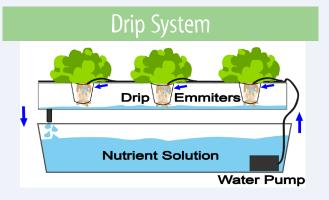
• **Drip** hydroponics can be set up for almost any type of plants you would like to grow. This system is rather simple: water is pumped in tubing to one or more plants; the nutrient-rich water then flows over the grow medium and drips down over the plant roots. Drip systems can be set up in either a recovery or a non-drip recovery method, depending on the reuse of the nutrient solution after it is dripped over the roots.
