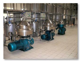
standardisation is usually combined with separation of the raw milk. Particularly, fat standardisation is used to control the fat content in various milk types. The more accurate the standardisation can be made, the better use of the costly fat. Here's an example: a producer is making 3% whole milk, yes, a milk intake on 300 tons milk per day. By accurate measurement he can move his production target by
